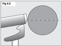
If using a skew chisel, the cutting edge should be applied approximately 3/8" (10 mm) above the centre height, see **fig 6.7**. A spindle gouge's cutting edge should come into contact with the workpiece approximately 3/8" (10 mm) below its centre, see **fig 6.8**.
